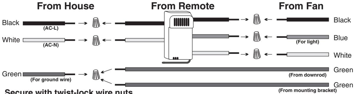
**Secure with twist-lock wire nuts.**
