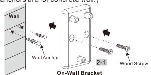
2-2. Snap the Hand-Held onto the On-Wall Bracket by aligning 3 posts to three recessed holes in back of Hand-Held.
