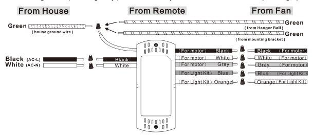
"Special note: All Green grounding wires, from <u>Hanger ball/Mounting bracket/Receiver</u>, must be well attached to House Ground/Earth to prevent flickering of LED."
