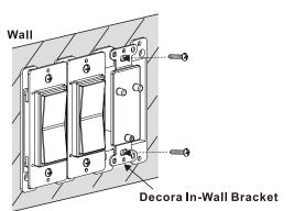
3-6. Install the wall plate onto the switch box and attach the screws removed from step 3-1.
