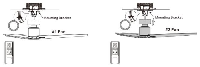
6 - 6. Switch on the main power and now each of these two fans are operated by its own remote individually.
