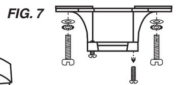
2. Remove one canopy screw (also Fig 7) and loosen the other. Make sure all of the wires are accessible and are not being pinched. Also, make sure the bracket doesn't wobble.
