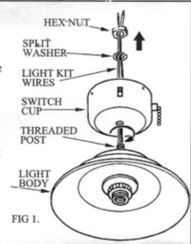
6. Insert the stripped ends of BLOCK the light kit's wires into the fan's light kit terminal block. White from the light kit to White from the fan. Black from the light kit to Blue from the fan. Tighten the set screws against the wire ends using the included screwdriver.
