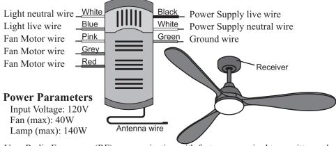
Uses Radio Frequency (RF) communication with factory pre-paired transmitter and receiver, that allows for one million possible unique pairs.
